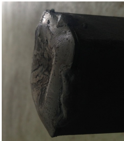
Post load image of capping domed plate failure mode
