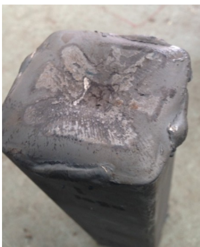
Post load image of capping domed plate failure mode
